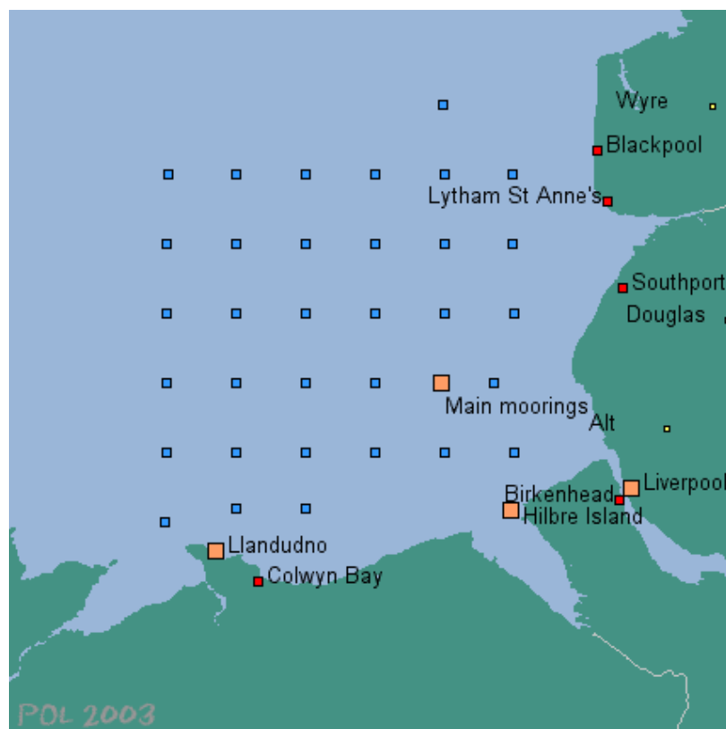
Liverpool Bay and the Coastal Observatory: blue squares are regular CTD stations, yellow squares are fixed moorings or coastal tide gauges.
